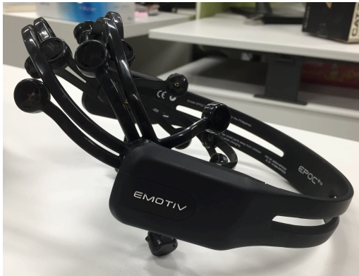
Fig. 1 EPOC+ which used for recording EEG in the experiment.
