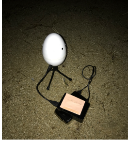
Fig. 6. Raspberry Pi 3 Model B with an 8-channel microphone array (TAMAGO-03)
