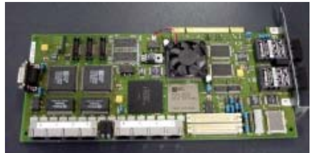
Figure 2: ENP-2505: IXP1200 evaluation board
