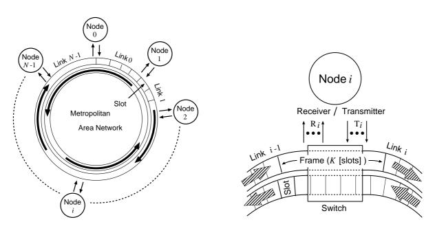
Fig. 2. A bidirectional ring with optical compression TDM
