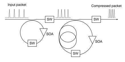
Fig. 1. Optical packet compressor
